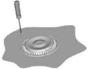
Fig. 1: Existing Drain Cover
